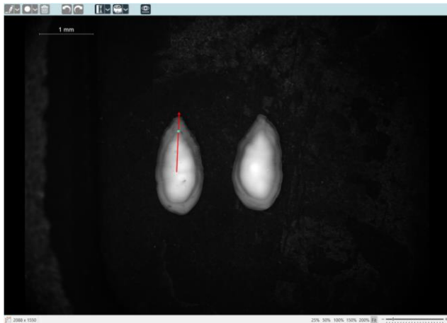
Figure 4: Sandeel_2022_034, modal age 0, catch date 21-11-2018, TL 100mm. Disagreement between readers on whether the innermost translucent zone should be counted as a winter ring or not. R01 NO and R03 DK estimating age 0.
